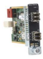
The Metrobility® Multi-rate Line Card (MRLC) by Telco Systems provides a transparent interface for multimode, singlemode, BWDM (single-strand bi-directional wavelength division multiplexing), and CWDM across a wide range of protocols with data rates ranging from 44.7Mbps to 2.7Gbps.
