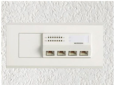
Micro Switch with cover installed in a hollow wall socket
