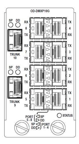
The 10G muxponder provides two trunk ports using OTN2 with FEC between a pair of OD-DMXP10G modules for a highly-reliable point-to-point link. The eight module access ports support several Ethernet and SONET protocol options. Other protocols and applications may be added in future updates.
