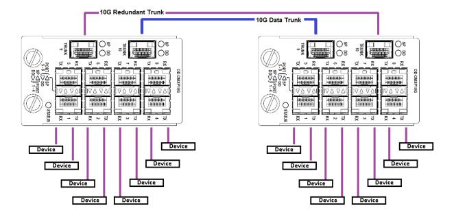
The example above shows local device connections at each end. Any of these individual devices could be intermediate network routing devices to further distribute the architecture.
